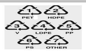
NOTE: PET-Polyethylene terephthalate, HDPE-High density polyethylene, V-Vinyl (PVC), LDPE- Low density polyethylene, PP-Polypropylene, PS-Polystyrene and Other means all other resins and multi-materials like ABS (Acrylonitrile butadiene styrene), PPO (Polyphenylene oxide), PC (Polycarbonate), PBT (Polybutylene terephalate) etc.
